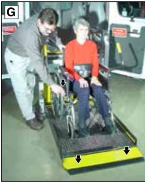
1. Read Notices below! Load passenger onto platform and lock wheelchair brakes. See Photo G.
