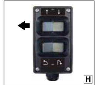
2. Press ↑ UP switch (Photo H) to fold roll stop UP fully (vertical - see Photo I), and raise the platform to floor level. See Photo J. Release switch.
